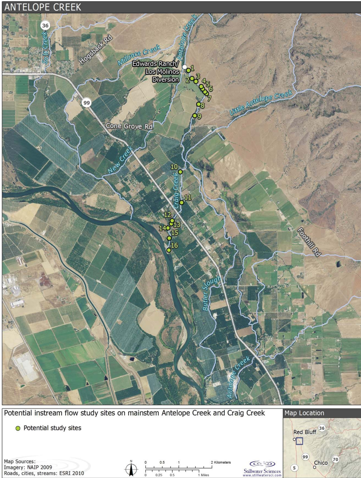
Figure 5-2. Potential instream flow study sites in mainstem Antelope Creek and Craig Creek.
