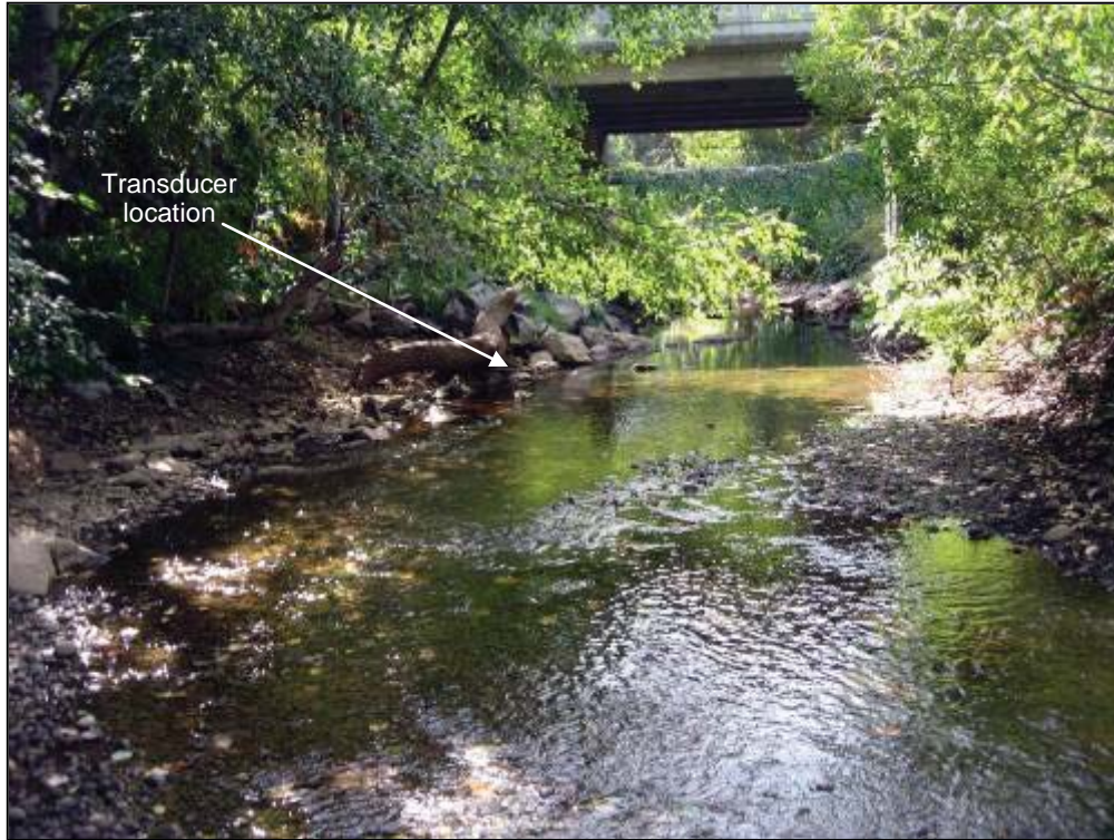
Figure C-66. Monitoring site 4 (Craig Creek at State Route 99) on 10 October 2010 showing summer baseflow at a water surface elevation slightly lower than the transducer.
