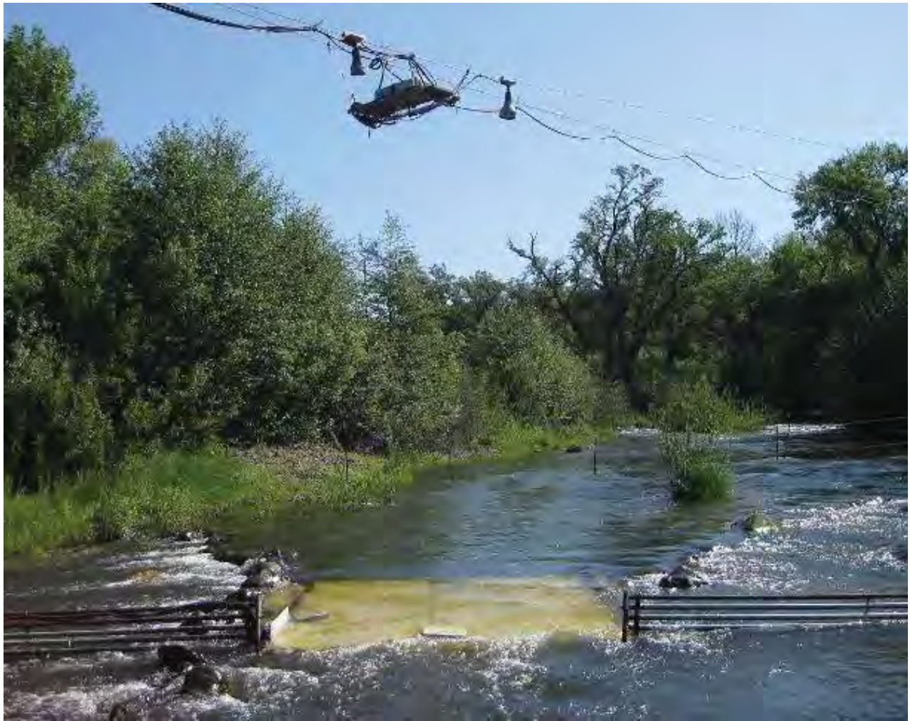
Figure 6. Camera box suspended over Bear Creek, looking upstream. Shown are three underwater cameras, the overhead camera, and the weir opening allowing fish passage.
