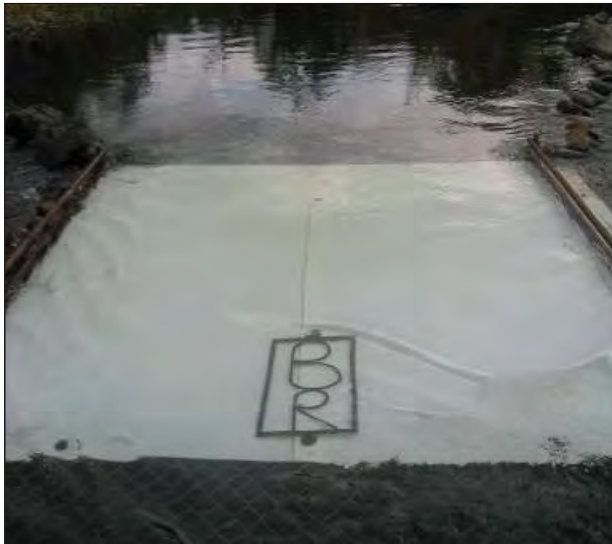
Figure 11. Two weir panels were added to the fish passage opening to prevent fish from skirting around the ends of the weir. A metal rectangle measuring 24 x 12-inches allowed tape readers to approximate fish lengths as well as identify the creek: BR= Bear Creek.
