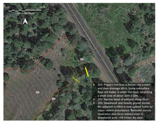
Figure 12: Detail Map of Area 6, Poppy's Fen, With the Intact Upstream Section to the Northeast of State Route 36E
